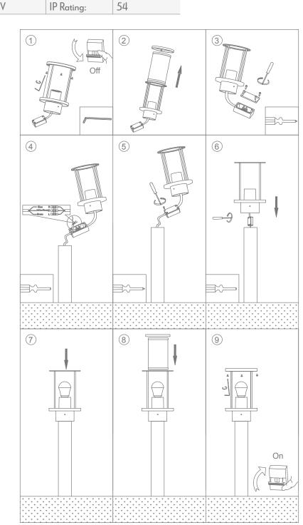
Note: -The lamp must be installed by professional electrician -Ensure the power supply is switched off before fitting this product
